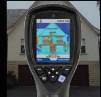
FLIR i3, temperature in 3,600 spots.
