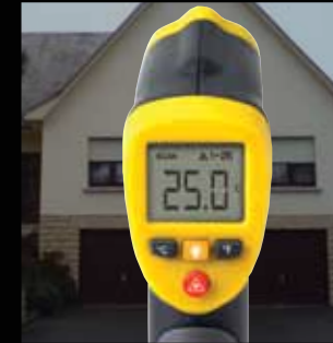
Spot pyrometer, temperature measurement in one spot.
